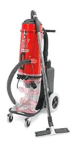
The Ermator S13 single motor Dust Extractor is available in 120V or 230V single phase. This powerful Dust Extractor is suitable for fine construction dust such as concrete grinding, building and plaster dust. It is equipped with a flushable fine filter and HEPA filters that meet asbestos standards.
