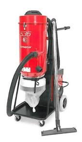
The S36 triple motor Dust Extractor is only available in 230V single phase. With its three large commercial-grade vacuum motors, it is the most powerful single phase dust extractor on the market today. What makes the S36 truly unique and unmatched in the concrete grinding and polishing industry is the quantity and size of its filters. It has a massive pre-filter with over 50-square feet of media, constructed in a cone-shape to reduce filter loading.
