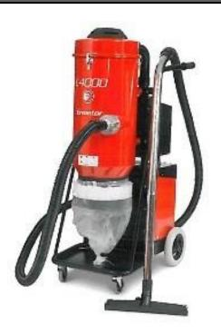
The T4000 (230 V) Three-Phase Hepa Dust Extractor is one of the newest members of Ermator's T-line. The 230V, 3-phase motor provides 280 CFM and 125" of water lift. The high water lift secures high suction secures high suction power to small and mid-size, low voltage concrete grinders, scarifiers, saws and shot blasters.
