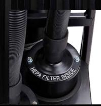
**3-step filtration**Dust extractors effectively separate the dust into three steps with a whirler, primary filter and HEPA H13 filter.
